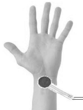
Fig 4. Force Sensor FSR-402 placed over the radial artery [1]
