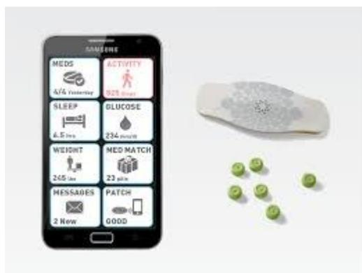
This disposable patch is worn on the body to capture and relay the body's physiological response and behaviors. In addition to recording information from the sensor, the patch records heart rate, temperature, activity, and rest patterns. The patch lasts approximately 7 days and is operated by a battery, which also lasts approximately 7 days. A mobile device is then carried in the pocket or purse to display data in context and support care.
