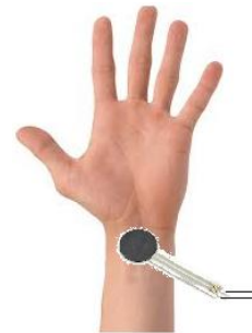
Fig 4. Force Sensor FSR-402 placed over the radial artery
