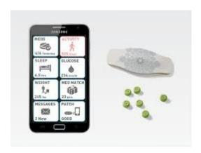
This disposable patch is worn on the body to capture and relay the body's physiological response and behaviors. In addition to recording information from the sensor, the patch records heart rate, temperature, activity, and rest patterns. The patch lasts approximately 7 days and is operated by a battery, which also lasts approximately 7 days. A mobile device is then carried in the pocket or purse to display data in context and support care.
